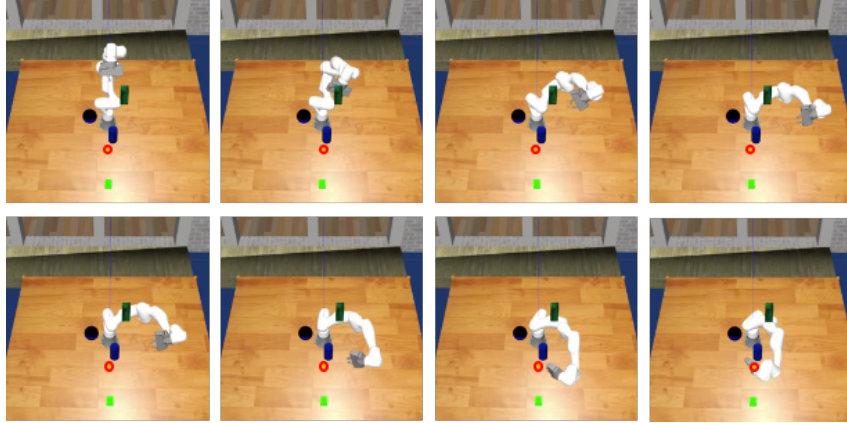
Figure 2: Multiple Obstacle Avoidance: Successful trial. The red circle is the goal.
