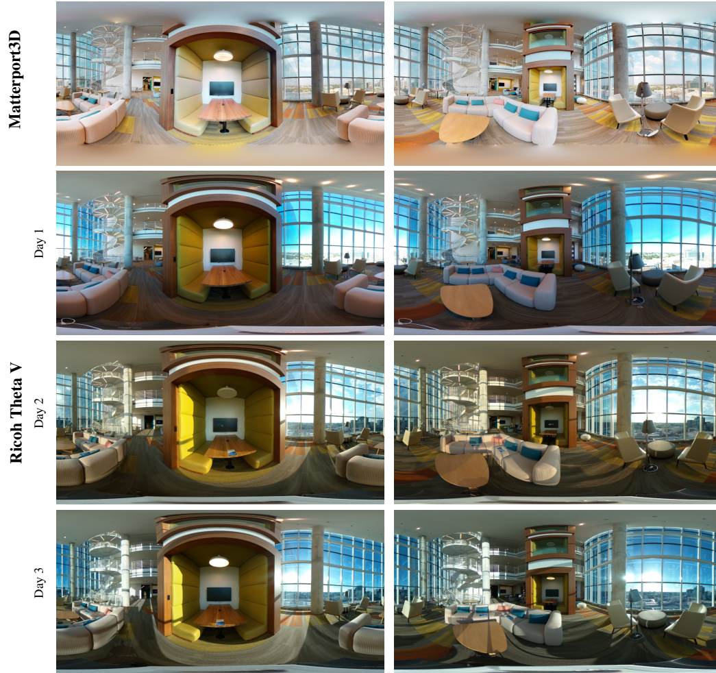
Figure 2: Panoramic captures in Coda from the Matterport3D camera (row 1) and the smaller and cheaper Ricoh Theta V camera (mounted on the robot) collected on three different days (rows 2-4). The robot camera’s limited dynamic range and loss of detail as compared to the Matterport3D camera (used for training the VLN agent) is clearly evident. Images collected on different days (with the robot camera) illustrate the variations in shadows, lighting, and precise object placement that confront the robot in the real physical environment.
