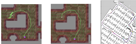
Figure 5: Navigation routes for two learned policies in the simulator (left: Lagrangian, middle: SDDPG- a ), and on-robot experiment of SDDPG- a (right).
