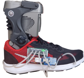
Figure 3: The Odyssey battery-powered lower-limb prosthesis which is actuated at the ankle. The Odyssey prosthesis is commercially available through SpringActive inc. [Link] .
