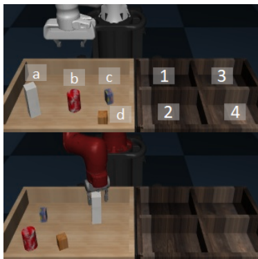
Figure 3: Our base environment is adopted from RoboTurk [51]. The 16 tasks consist of taking an object (a-b) to a bin (1-4). Top robot is agent and bottom is demonstrator.
