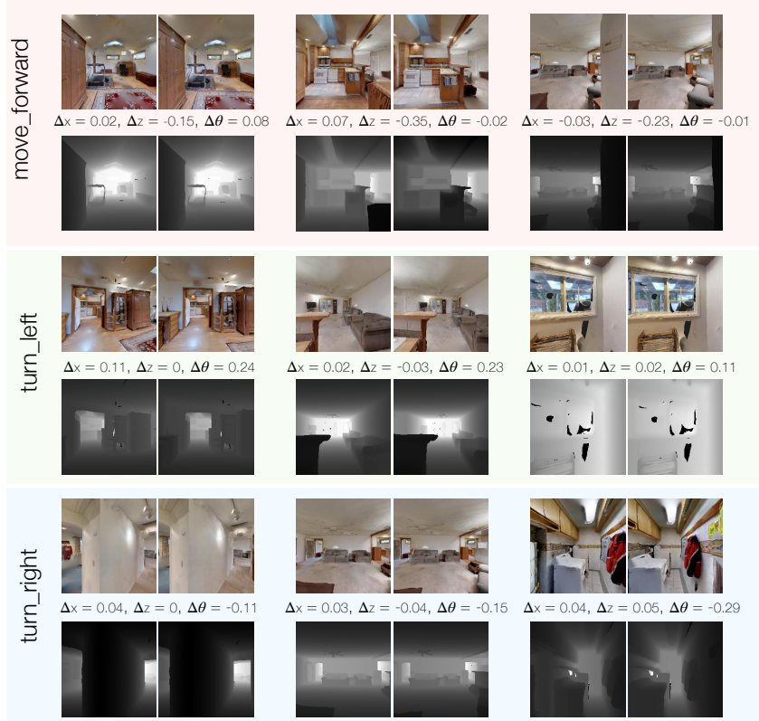
Figure 5: Visualization of samples from the egomotion dataset collected in a noisy actuation setting. We group the data points according to the action – move-forward, turn-left and turn-right. For every data point, we show the RGB image frames, depth maps and the relative pose change between the source and target agent states.
