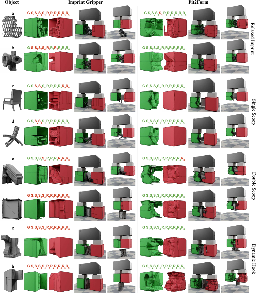
Figure 5: Qualitative Results. We compare with grippers generated using the Imprint baseline and highlight four typical strategies used by Fit2Form: relaxed imprint (a,b), single-sided scoop (c,d), double-sided scoop (e,f), and dynamic hook (g,h). The green/red string above each gripper indicates success/failure of grasp success, 4 stability, and 6 robustness metrics. Objects in b,e,g,h adversarial objects from DexNet 2.0, the rest are from ShapeNet.
