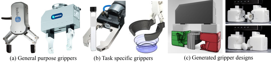
Figure 1: Robot Gripper Design. While most of the recent works have been focused on learning robust control policy for general-purpose grippers (a), the majority of robot grippers in industrial applications are highly customized to improve the system’s robustness and accuracy for the target task (b). However, the process of manual hardware design is costly and time-consuming. The goal of Fit2Form is to automate this design process with a data-driven approach and generate gripper geometry for a target object that would satisfy the design objectives (c).
