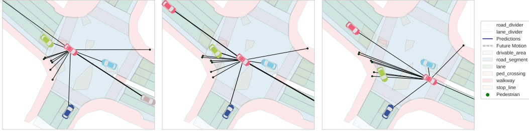
Figure 4: The B matrix allows us to infer the influence that the ego-agent (red vehicle crossing the intersection) has on other agents. Line thickness is determined by the Frobenius norm of the corresponding block in the B_z matrix of the most-likely mode z . As can be seen, when the ego-vehicle is in the middle of the intersection it is maximally influencing the other vehicular agents, and less so before and after being in the intersection. Pedestrians are equally influenced through time.
