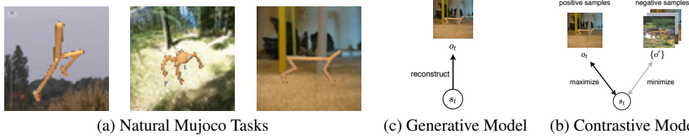
Figure 1: (a) CVRL addresses the tasks of sparse rewards, many degrees of freedom, and complex observations. (b) Standard generative observation model learns an observation likelihood function p(o_t | s_t) , i.e., reconstructing observations o_t from s_t , which includes the irrelevant background features. (c) CVRL discovers the correspondence between state s_t and observation o_t by maximizing their mutual information I(s_t, o_t) by scoring the real pair (s_t, o_t) against fake pairs \{s_t, o'_t\} , which avoids pixel-level reconstruction.
