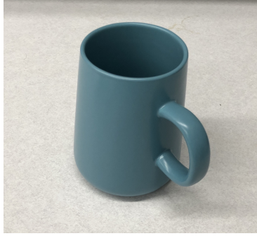
Figure A6: The only mug failed to be grasped during one set of trials. It has a unique shape with a larger diameter at the bottom than at the rim.
