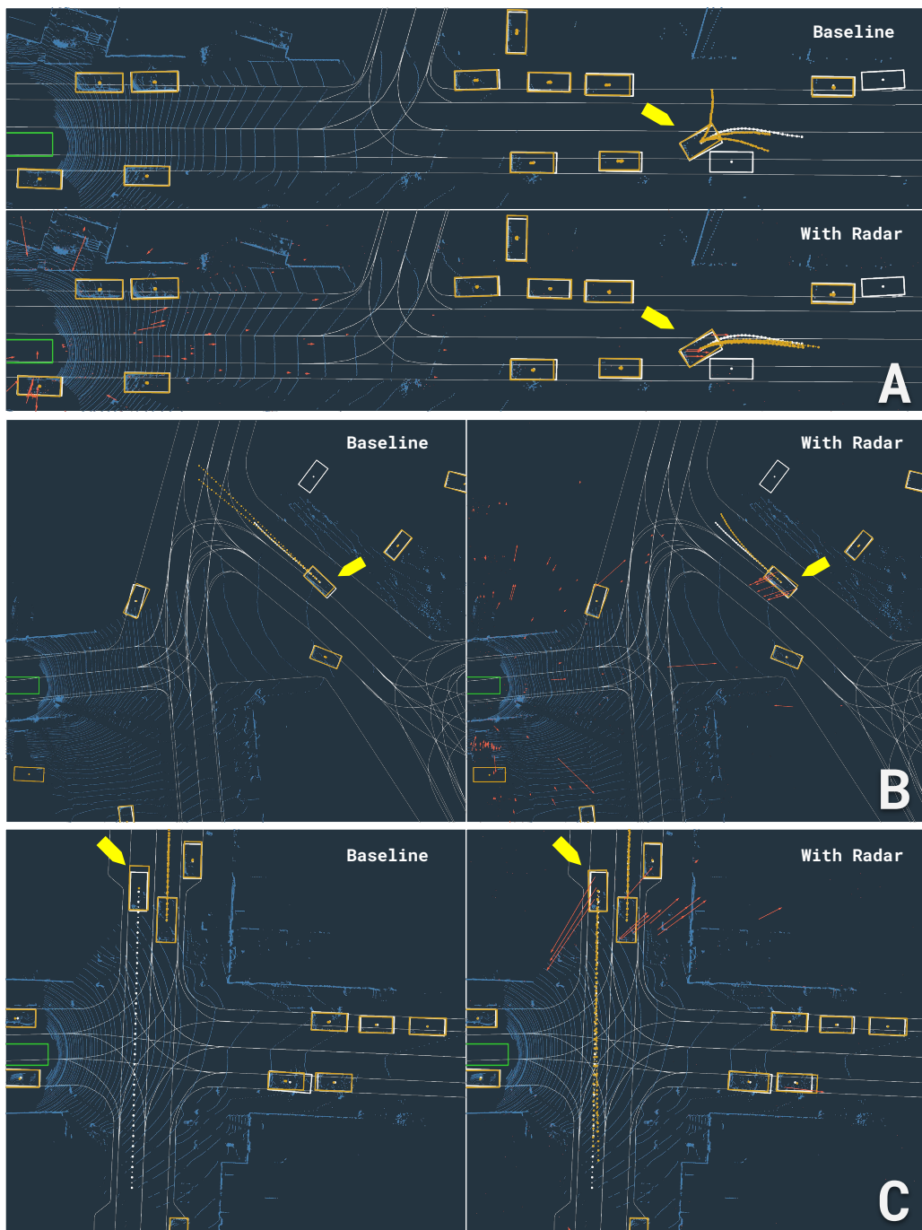
Figure 3: Improvements in Prediction. These three scenes show where radar improves trajectory prediction. The vehicle in A is accelerating into the street. Given the range and high acceleration of the vehicle, radar shows a clear benefit in estimating object trajectories with respect to the lidar only baseline. Similarly, B shows a case where the addition of radar helps accurately predict the motion of a vehicle slowing down for a turn. In C a vehicle has just come from an area of occlusion resulting in sparse historical lidar data. The radar data lets the model quickly estimate an accurate future trajectory.
