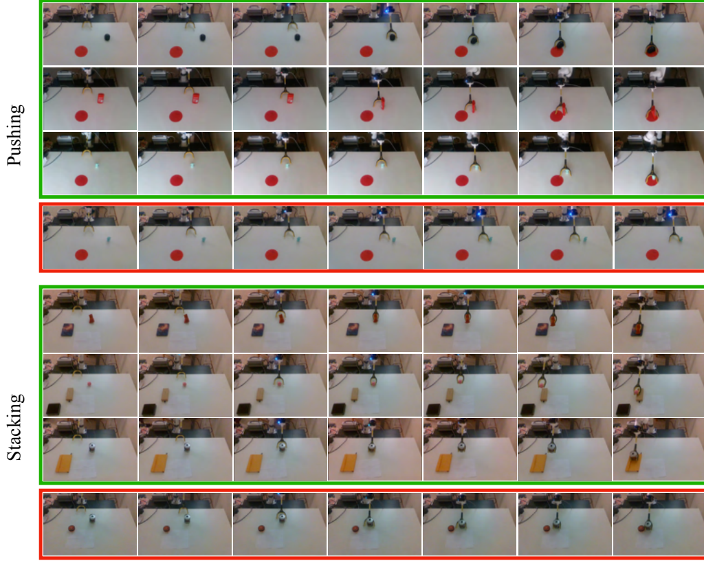
Figure 10: We visualize additional trajectories executed on the robot using our learned pushing and stacking policies from a third person point of view. Successful trajectories are highlighted in green, unsuccessful ones in red.
