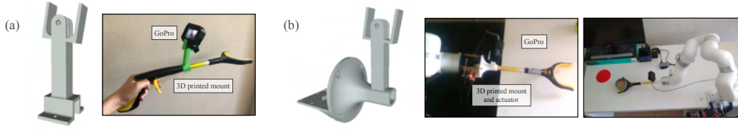
Figure 7: In part (a), we show the setup for collecting human demonstrations. This includes a 3D printed mount, a camera, and the reacher-grabber stick. Part (b) displays the corresponding setup on the robot.
