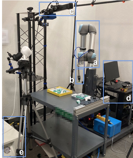
Figure 12. Hardware setup. a) UR5e Robot, b) Piab suction cup, c) Photoneo camera, d) Linux PC, and e) air compressor and vacuum generator.
