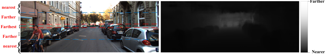
Figure 3: Depth distribution in monocular images.
