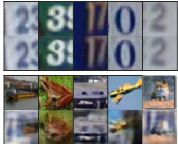
Figure 7: AMA trained on SVHN data: Here we show the performance of the model on test time SVHN images vs anomalies coming from CIFAR-10 dataset. Odd rows represent ground truths, and the even rows show the reconstructions. Similar to 6, the model performs well on normal test time samples, but reconstructs anomalies badly.
