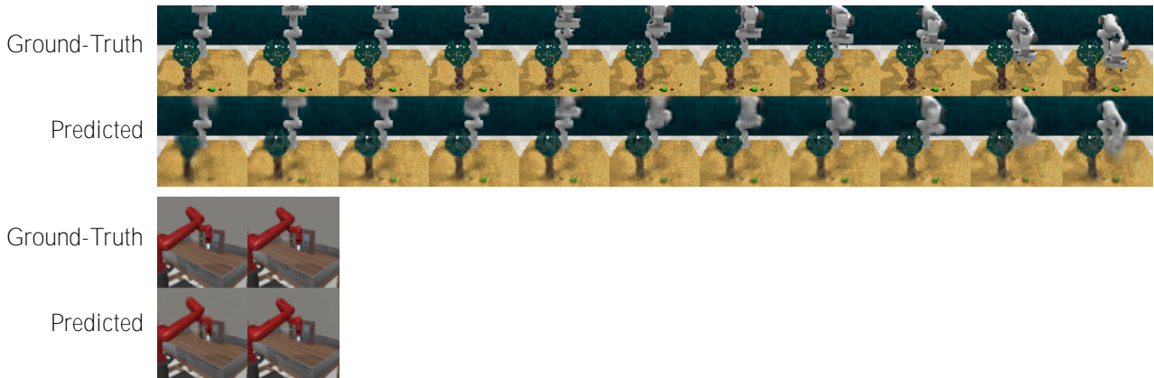
Figure 13. Future frames predicted by our action-free video prediction model on RLbench (top) and Meta-world (bottom). We observe that predicted frames on both datasets capture dynamics information of robots (e.g., how robots are moving towards objects), while prediction in RLbench is not high-quality as in Meta-world which is a more simple domain.
