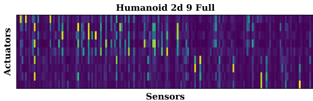
Figure 7. Visualization of the cross attention weights in the final layer of our policy model on the Humanoids task and Humanoid 2d 9 Full morphology. Each cell in the attention matrix corresponds to the maximum attention value for that cell over an entire episode. Cells with dark shading indicate that our model ignores those sensors over an entire episode by zeroing their attention weights.
