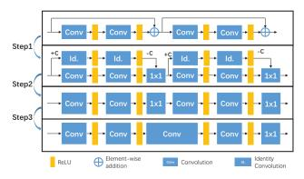
Figure 3. Illustration of converting general models to plain networks. ReLU activation functions in the figure can be replaced with any activation function that preserved the non-negative value. C is the large constant mentioned in Proposition 3.6. Step1: Convert the skip connection into 1×1 convolutions. Step2: Merge the convolutions with different kernel sizes. Step3: Merge neighboring 1×1 convolution and following convolution.
