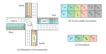
Figure 1. An illustration of intersection, traffic movements and traffic signal phase.
