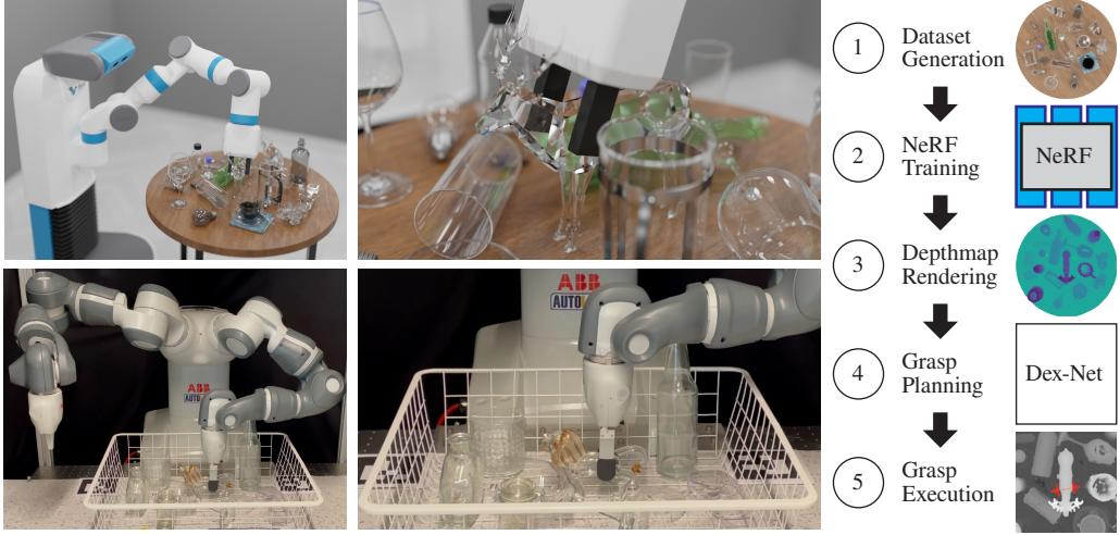
Figure 1: **Using NeRF to grasp transparent objects** Given a scene with transparent objects (left column), we the pipeline on the right to compute grasps (middle column). The top row shows Dex-NeRF working in a simulated scene while the bottom row shows it working in a physical scene.
