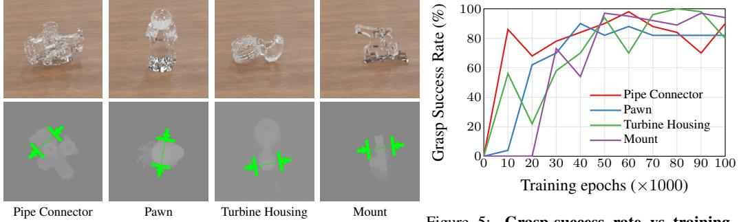
Figure 4: **Synthetic singulated objects** used in simulation experiments. **Top row:** image of the object in the training data. **Bottom row:** computed depth map and candidate grasp.
