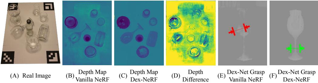
Figure 3: **Using NeRF to render depth for grasping transparent objects.** Dex-NeRF uses a transparency-aware depth rendering to render depth maps that can be used for grasp planning. In contrast, Vanilla-NeRF’s depth maps are filled with holes and result in poor grasp predictions.
