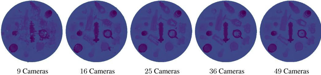
**Figure 9: Depth rendering using a grid of overhead cameras.** Using increasing amounts of overhead cameras improves the quality of the depth map and its utility in grasping, however, beyond a certain number of cameras there is a diminishing return.
