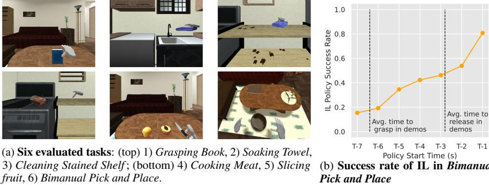
Figure 5: **Evaluation:** We create six novel household tasks in iGibson 2.0 where the agents have to manipulate extended states. These tasks cannot be studied in other simulation environments.
