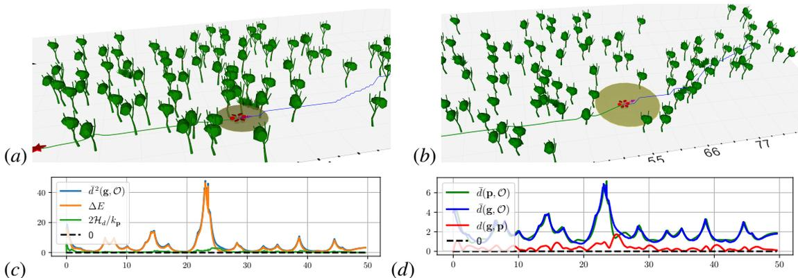
Figure 4: Safe navigation of a hexarotor robot in a forest is demonstrated in (a) and (b). The bottom plots (c) and (d) show the dynamic safety margin  $\Delta E$ , the scaled desired Hamiltonian  $2\mathcal{H}_d(\mathbf{x}, \mathbf{x}^*)/k_p$ , and the distance to the obstacles  $d(\mathbf{p}(t), \mathcal{O})$ , indicating that the safety constraints are never violated.
