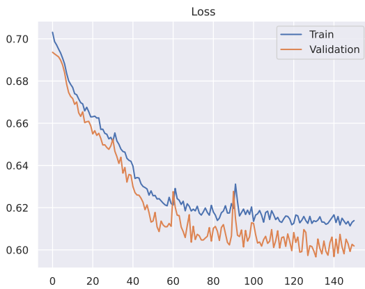
Figure A.12: Loss for our encoder trained on the HiRID data. A couple of the loss spikes caused by dimension pruning can be observed (at epochs 60 and 90)
