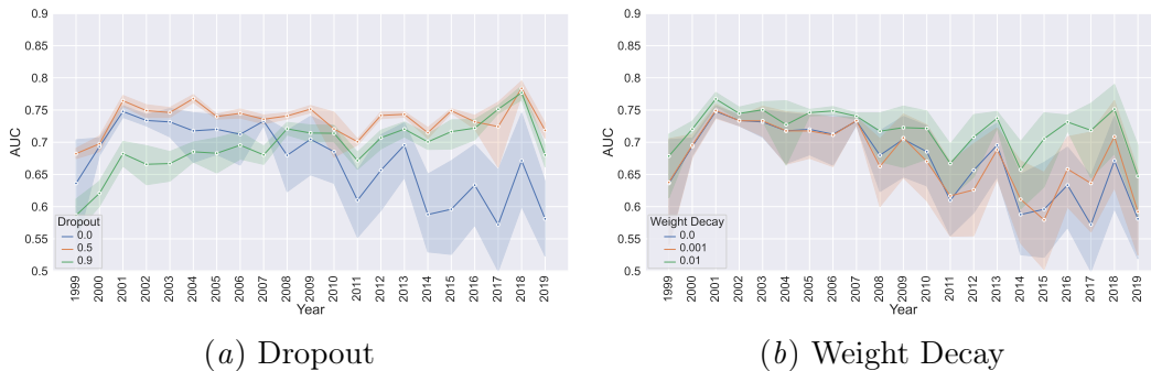
Figure 5: Effect of regularization on error amplification strength on MIMIC-IV data for a four hidden layer network with an initial FPR of 0.2. Both dropout and weight decay are highly effective at reducing error amplification, and improving initial model performance, with dropout performing slightly better.
