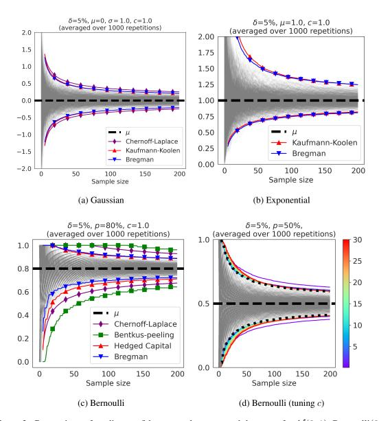
Figure 2: Comparison of median confidence envelopes around the mean for  $\mathcal{N}(0,1)$ , Bernoulli(0.8) and  $\mathrm{Exp}(1)$ , as a function of the sample size n, over 1000 independent replicates. Grey lines are trajectories of empirical means  $\widehat{\mu}_n$ . Bottom right: confidence envelopes for varying regularization  $c \in [0.1, 30]$  for Bernoulli(0.5) distribution. Dotted black line: heuristic  $c_n \approx 0.12n$ .
