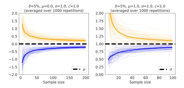
Figure 3: Examples of confidence upper and lower envelopes around unknown expectation  $\mu=0$  for  $\mathcal{N}(\mu,1)$  (left, cf. Table 2) and unknown standard deviation  $\sigma=1$  for  $\mathcal{N}(1,\sigma)$  (right, cf. Table 2), as a function of the number of observations n. The thick lines indicate the median curve over 1000 replicates.
