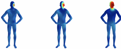
Figure 2: Wavelets on the FAUST dataset with g(\lambda) = e^{-0.0005\lambda} , j = 1, 3, 5 from left to right. Positive values are red.
