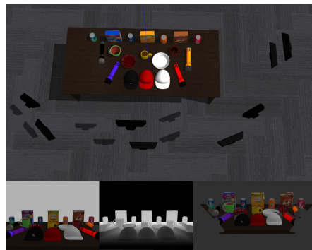
Figure 3: Synthetic recreation of a tabletop scene in Gazebo. The object catalogue (top), an example front view RGB (bottom-left) and depth (bottom-middle) pair, as well as the corresponding point cloud visualized in RViz (bottom-right).
