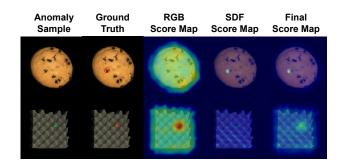
*Figure 1.* Results of our method on the MVTec 3D-AD dataset. Defects that are only perceptible in one but not the other modality can be successfully localized by our method.
