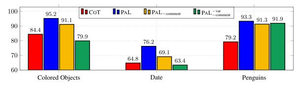
Figure 9: Ablation study of PAL prompt formats. We consider the original PAL prompt, it with natural language comments removed ( $PAL_{comment}$ ), and further variable names replaced with random character ( $PAL_{comment}^{-var}$ ). As a reference, we also show the CoT performance (blue).
