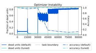
Figure 1. Abrupt task changes can drive instability in optimizers which depend on second-order moment estimates for adaptive learning rate scaling. Setting these estimators to be more robust to small gradient norms and to update moment estimates more quickly mitigates this issue.
