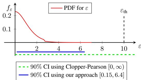
Figure 1. Comparison of the posterior PDF  $f_\epsilon$  using our Bayesian approach and the upper bound  $\epsilon_{th}$  obtained from a state-of-the-art DP accountant (Gopi et al., 2021) for a CNN trained on CIFAR-10 with  $\delta$  of  $10^{-5}$ . Empirical evaluation suggests stronger privacy than what can be proven using accountants. Below the plot, we illustrate the reduction in uncertainty of the 90% credible interval of our Bayesian approach over Clopper-Pearson intervals.
