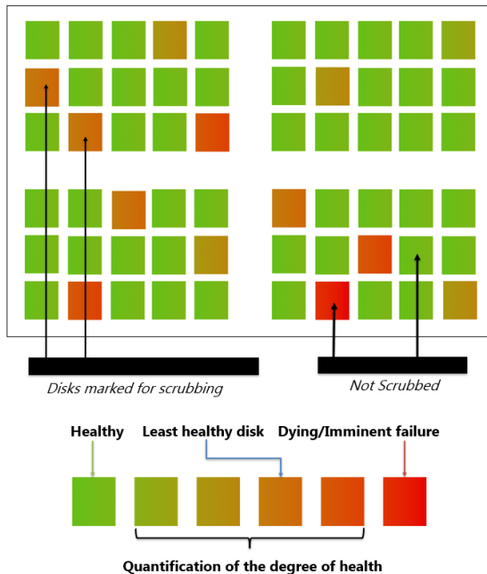
Figure 2: Quantifying the health of disk drives: The disks which are healthy and non-healthy are not selected for scrubbing, while the disks of concern are marked for scrubbing.
