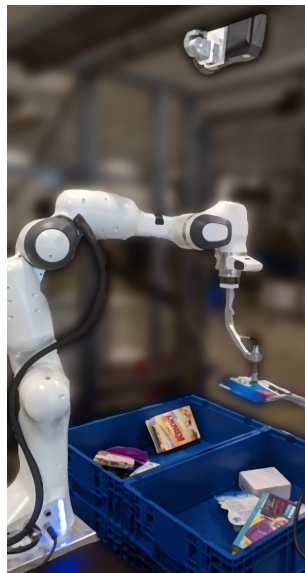
Figure 1: Bin-picking setup with a single, fix-mounted overhead camera.
