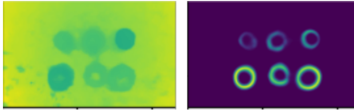
Figure 2: Heatmap output for objects including upside-down glasses. In this scene the top 3 objects are upside-down (and hence ungraspable) and the bottom 3 are graspable. The left image shows depth rendered from NeRF and the right image shows the location heatmap output by Rad-Net. Note how the heatmap activates much less on upside-down objects (<15% confidence) compared to graspable glasses (80% confidence).
