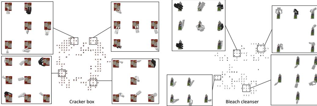
Figure 1: Barnes-Hut t-SNE visualization [9] using our learned embeddings of grasps from five different robotic hands.
