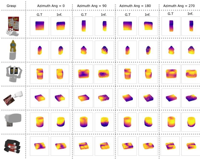
Figure 3: Multi-view visualization of ground truth (G.T) and inferred (Inf.) contact maps across different grippers and objects. Brighter regions correspond to the contact regions.
