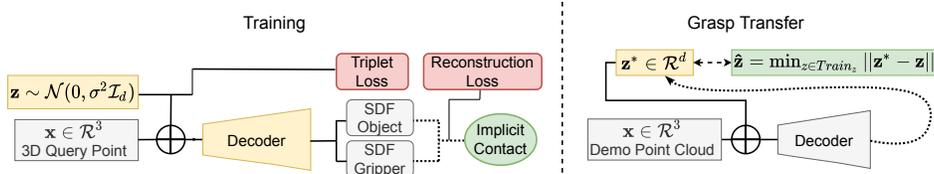
Figure 2: Left) Our network architecture with the training losses. Right) Illustration of the grasp transfer process during inference. Yellow modules indicate trainable parameters.
