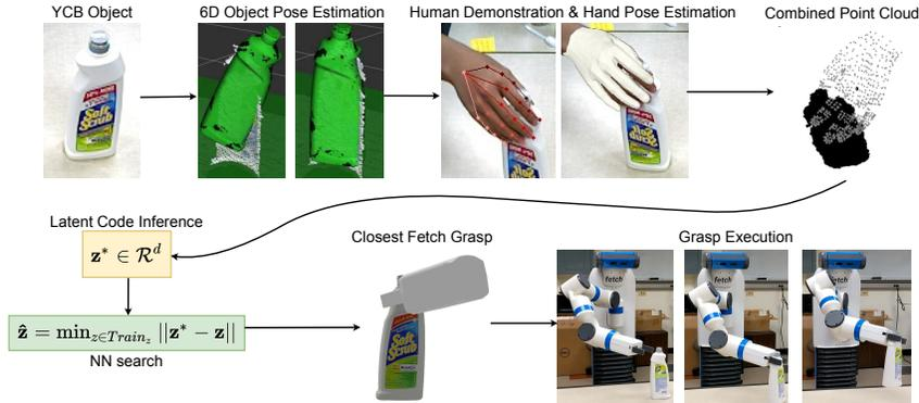
Figure 6: Our pipeline for grasp transfer from human demonstrations to a Fetch mobile manipulator.
