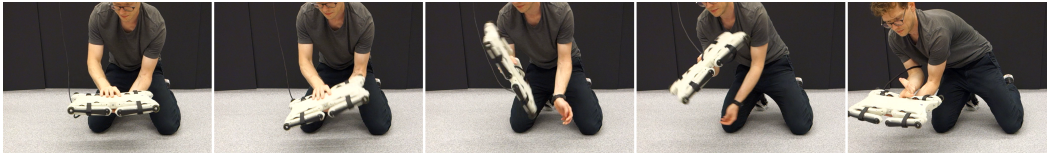
Figure S1: Hand-held motion demonstration for SOLOBACKFLIP. Note that the robot joints are not actuated and only base information is recorded.
