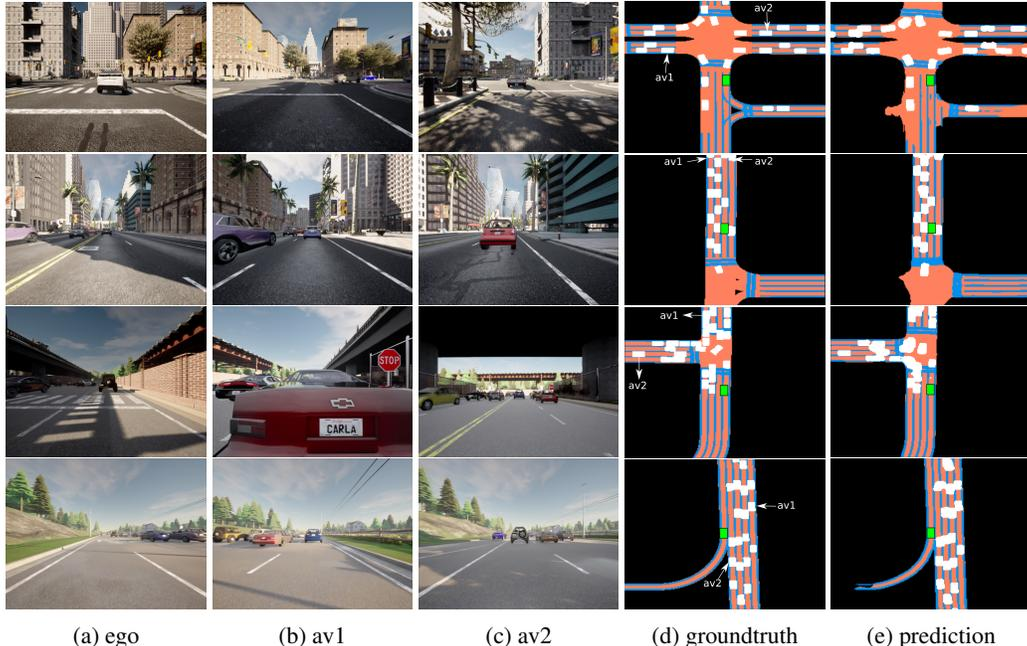
Figure 4: **Qualitative results of CoBEVT.** From left to right: the front camera image of (a) ego, (b) av1, (c) av2, (d) groundtruth and (e) prediction. The green bounding boxes represent ego vehicle, while the white boxes denote the segmented vehicles. CoBEVT demonstrates robust performance under various traffic situations and road types.
