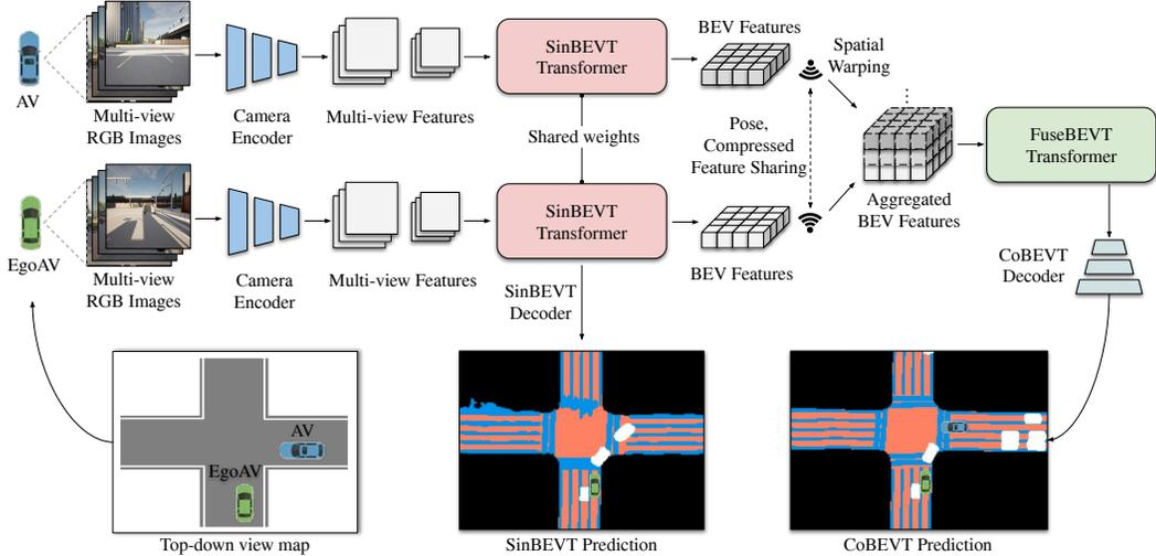
Figure 1: The overall framework of CoBEVT.
