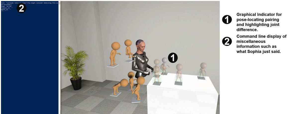
(b) Close view of the wizard's monitor screen where critical information of the posing task's execution is displayed.
