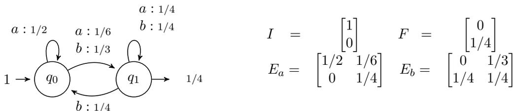
Figure 2: An automaton in its graphical form and its equivalent linear representation.
