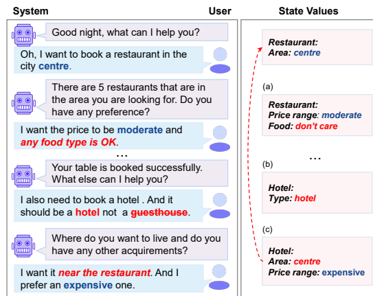
Figure 1: Three main issues of state value generation in DST: (a) “ don’t care ” should be generated, (b) “ hotel ” should be distinguished from “ guesthouse ”, and (c) “ centre ” should be inferred from the first turn. Words in blue are state values that can be extracted directly.
