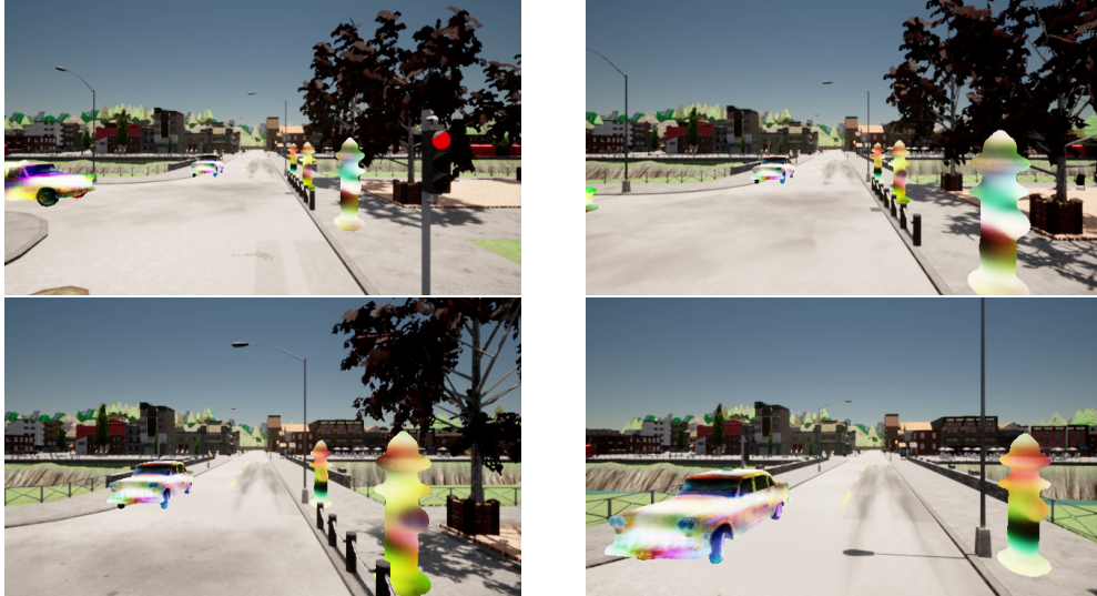
Figure D.2: Sample renderings of the left turn trajectory with the adversarial perturbations in CARLA from the ego vehicle’s point of view. Four different snapshots from the evolution of the trajectory are shown.
