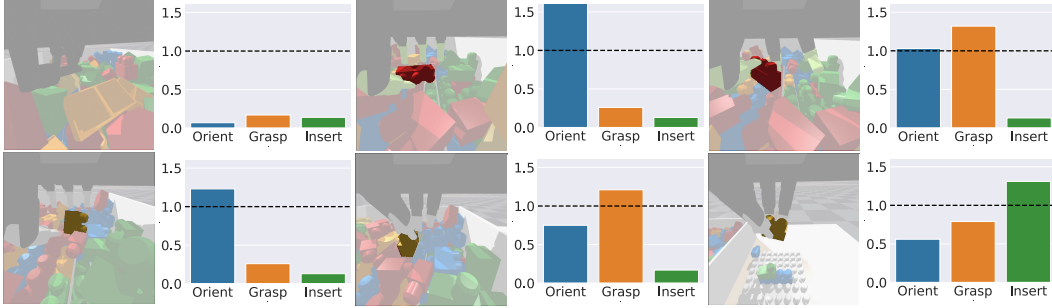
Figure 4: Examples of policy-switching with transition feasibility function. Each example contains an image from the wrist-mount camera (left) and its corresponding feasibility score c_i outputted by the transition feasibility function (right). We highlight the target block in the image for better visualization. The policy-switching process visits each sub-policy in reverse order. The first sub-policy with a feasibility score c_i > 1.0 is selected for execution.
