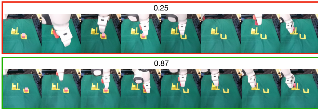
Figure 5: Demo Quality Estimation. We show the predicted quality for real-world demonstrations of the Stack task. The trajectory segments with less optimal behaviors (e.g., jittering or waving) will be assigned with lower scores (marked with red bounding boxes).
