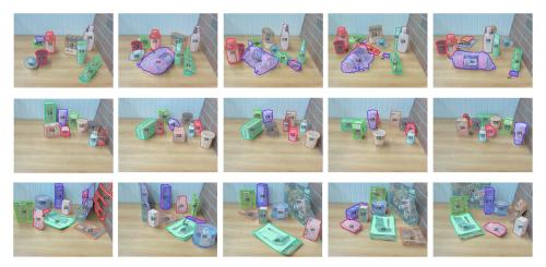
Figure 5: Visualized results for the table environment. Masks with the same color and index are associated and predicted as the same object by the network.
