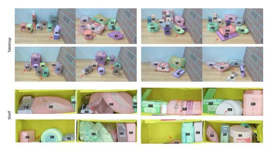
Figure 10: Failure Cases Illustrated. In the Tabletop settings (top 2 rows), we observe under-segmentation (top left), over-segmentation (top right), mismatch (bottom left), and mistrack (bottom right). In the Shelf settings (bottom two rows), the failures include a combination of under-segmentation and failure to detect new objects (top left), failure to track and mismatch (top right), failure to detect (bottom left), and failure to segment (bottom right).
