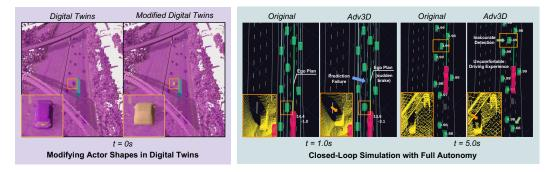
Figure 1: ADV3D is a framework that evaluates autonomy systems in closed-loop on complex real-world scenarios, and alters the scene appearance via actor shape modification (left) to create more challenging scenarios that cause autonomy failures such as inaccurate detections, incorrect predictions and strong decelerations or swerving, resulting in uncomfortable and dangerous maneuvers (right).
