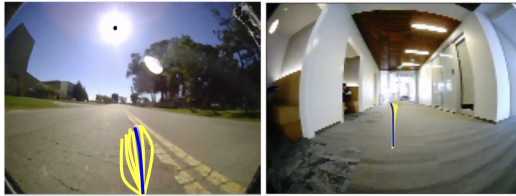
Figure 9: ViNT exhibits an implicit preference for following paved roads ( left ) and hallways ( right ).
