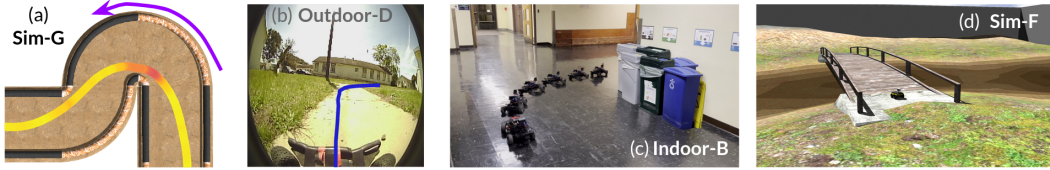
Figure 5: Emergent behaviors with FastRLAP. Maximizing speed with RL results in a “racing line”, braking as late as possible to maintain speed in and out of tight corners (a) and drifting on slick surfaces (c). Outdoors, tall grass slows the robot’s motion, promoting driving on paths (b). In Sim-F , the robot infers that the bridge is faster than driving through mud via visual correlation (d).
