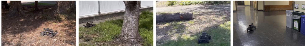
Figure 2: FastRLAP learns fast driving policies for a 1/10 th -scale vehicle operating in diverse indoor and outdoor environments with challenging terrain in tens of minutes, using offline pre-training and online RL.
