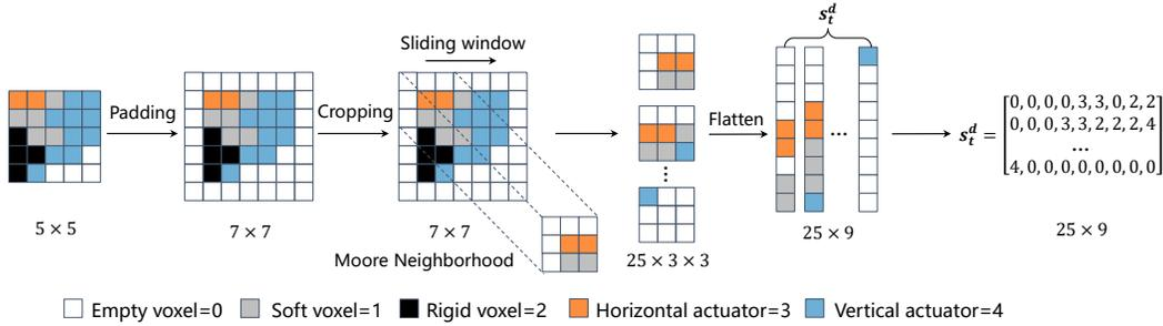
Figure 5: Parameterization of the design space. Initially, the design space is surrounded by empty voxels. Each voxel is denoted by a discrete value, reflecting its material characteristic. Then, a sliding window is used to get each voxel’s local state, which is composed of its type and the types of its Moore neighbors. Finally, the design state is formulated as an ordered sequence.
