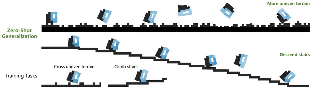
Figure 7: Visualization of PreCo’s zero-shot behavior. The figure shows screenshots at consecutive time intervals of the designed robot’s behavior. Compared with training tasks, We find that PreCo shows favorable generalization properties and intriguing behavior when facing new environments (beginning from 00 : 28 in this video).
