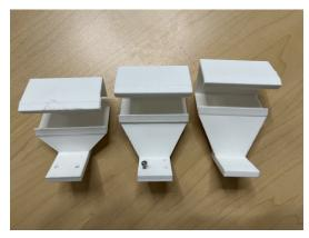
Figure 12: Our wrist camera mounts. The follow depicts the original, 35-degree and 50-degree mounts.
