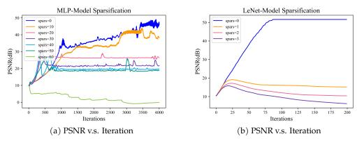
Figure 4: Performance (PSNR) comparison of applying model sparsification on (a) MLP network and (b) LeNet.
