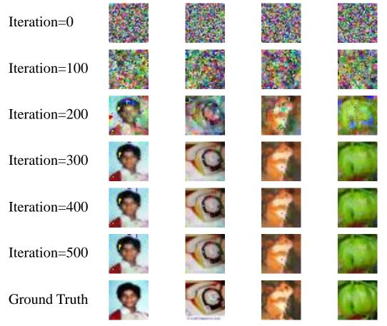
Figure 14: The LeNet restoration result of DLM+ for batch data. Approximately 300 rounds, the ground-truth image has been completely recovered.
