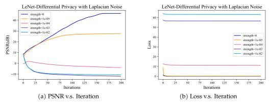
Figure 8: Performance comparison of applying differential privacy with various Laplacian noise strength to LeNet network.
