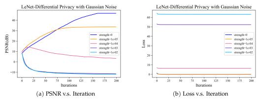
Figure 7: Performance comparison of applying differential privacy with various Gaussian noise strength to LeNet network.
