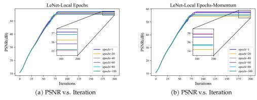
Figure 3: Performance (PSNR) comparison of LeNet with (a) SGD and (b) SGD with momentum under different local iterations.
